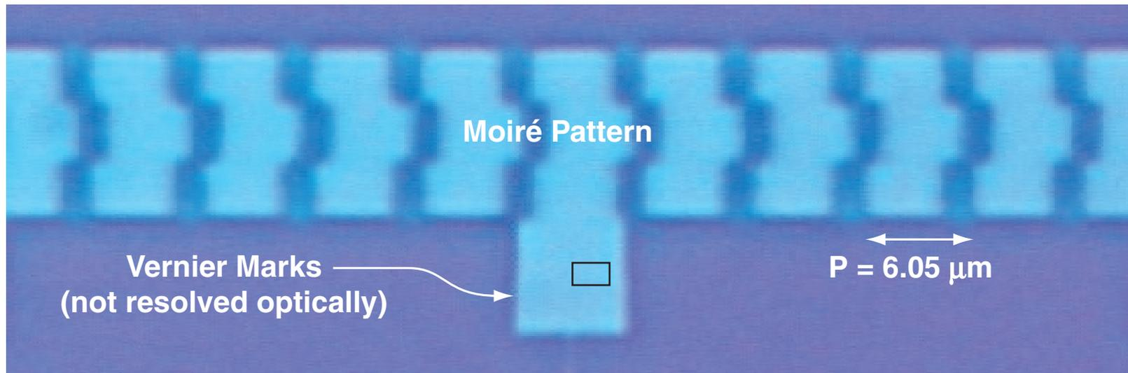
SEM of Vernier Marks (after liftoff of Chromium)
