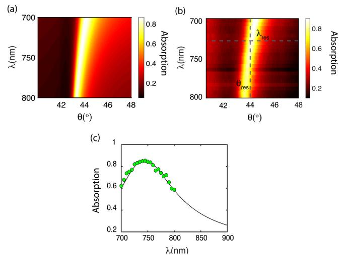
**Fig. S1.** (a) Simulation and (b) measurement absorption for the gold sample while coupling to the propagating surface plasmon for different incident wavelengths. In (c), the solid line (simulation) and dots (experiment) are extracted from the computed mesh plots in (a) and (b) at 745 nm resonance wavelength, respectively.
