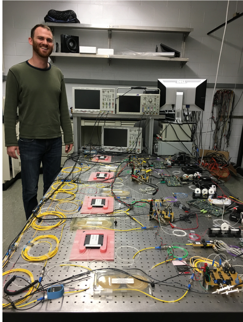
Figure 2.4: Photograph of our 4-node network of opto-electronic oscillators.
