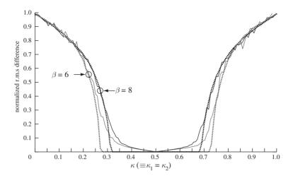
Figure 8. Measured and simulated normalized synchronization error as a function of  $\kappa$  for  $\beta = 6$  (grey lines) and 8 (black lines). The measurements (solid lines) and simulations (dotted lines) were conducted using symmetric bidirectional coupling, ( $\kappa_1 = \kappa_2 \equiv \kappa$ ).
