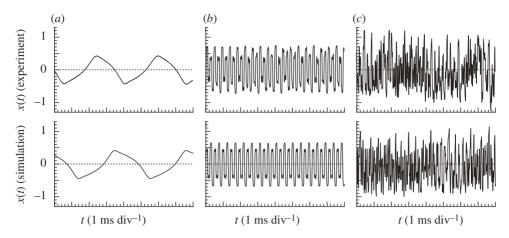
Figure 2. Typical measured and calculated time traces for the nonlinear opto-electronic oscillator system, for feedback strengths of (a)  $\beta = 1.5$ , (b) 3.0 and (c) 4.5.
