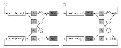
Figure 6. (a) Block diagram of two linearly coupled opto-electronic chaotic oscillators, where the coupling and delays are taken to be in the optical path connecting the two systems. (b) Equivalent system, obtained by commuting the coupling and delay with the band-pass filter. In practice, the coupling is implemented optically as in (a), but for convenience, we analyse the equivalent scenario depicted in (b).
