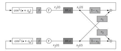
Figure 7. Block diagram of two diffusively coupled oscillators. The coupling is constructed in a way that guarantees that the resulting system admits a synchronous solution of the form  $x_1(t) = x_2(t) \equiv x(t)$ , where x(t) exhibits the same dynamical behaviour as that of an isolated system.
