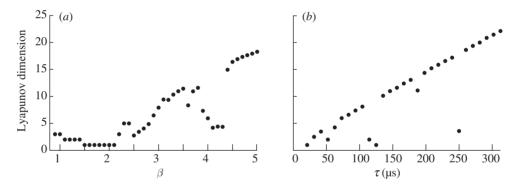
Figure 4. Calculated Kaplan–Yorke (Lyapunov) dimension: (a) as a function of the feedback strength  $\beta$ , for fixed feedback delay  $\tau = 230~\mu s$  and (b) as a function of the feedback delay  $\tau$ , for fixed  $\beta = 4.5$ . The remaining system parameters are given in table 1.
