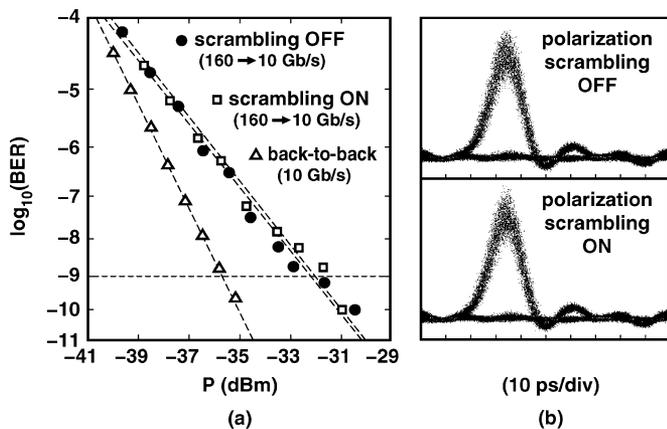
Fig. 3. (a) BER versus received power for the 160-Gb/s demultiplexer, showing little penalty when polarization is scrambled. (b) Measured eye diagrams of demultiplexed 10-Gb/s data, with and without polarization scrambling.
