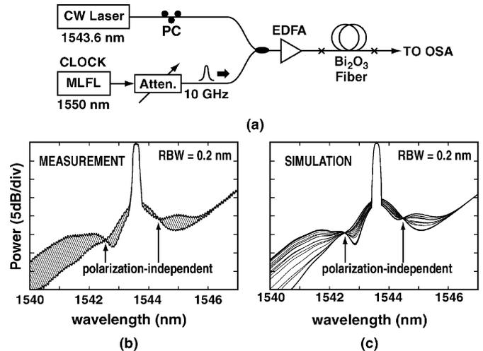
Fig. 4. (a) Experimental setup used for CW XPM measurements. (b) Measurement and (c) simulation of XPM-induced spectral broadening for different polarization states. The spectra appear tilted because of residual spectral power from the nearby pump signal (not shown).
