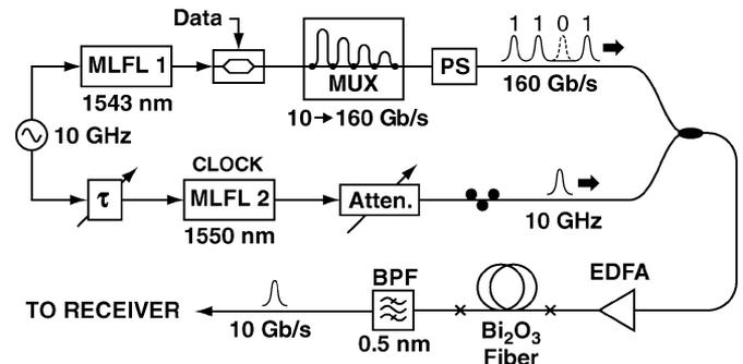
Fig. 1. Experimental setup used in polarization-independent 160-Gb/s demultiplexing. The polarization scrambler (PS) is used to evaluate the effect of polarization fluctuations.
