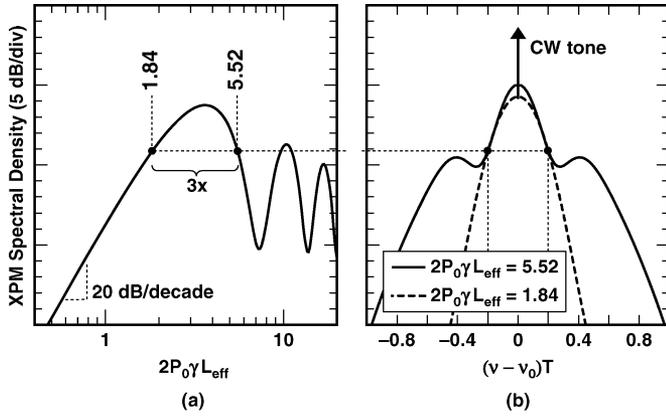
Fig. 5. (a) Calculated XPM spectral power at an offset frequency of  $(\nu - \nu_0) = \pm 0.2/T$ , as a function of  $2P_0\gamma L_{\text{eff}}$ . The two labeled points show that  $\gamma$  can change by  $3\times$  without changing the XPM spectral power. (b) Calculated XPM spectra for the two points labeled in (a), showing the crossing points at  $(\nu - \nu_0) = \pm 0.2/T$ .
