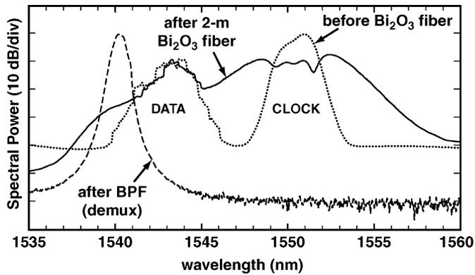
Fig. 2. Optical spectra before entering the fiber (dotted line), after 2 m of Bi<sub>2</sub>O<sub>3</sub>-based fiber (solid line), and after bandpass filtering (dashed line).
